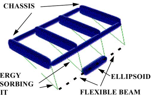
**Figure 4. Energy absorbing underrun barrier model**
