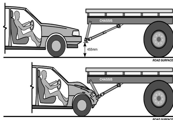
Figure 1. Illustration of the energy absorbing underrun barrier on the rear of a truck, before and after impact. [Rechnitzer et al 1996]
