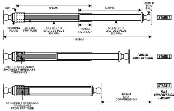
**Figure 2. Schematic diagram of an energy absorbing tube-in-tube struts. [Rechnitzer et al 1996]**
