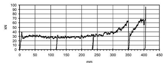
**Figure 5. Force deformation curve for the static compression test of the energy absorbing unit**
