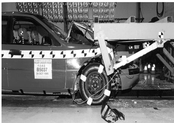
**Figure 3. Photograph of a vehicle in a 48kph impact with an energy absorbing barrier. [Rechnitzer et al 1996]**
