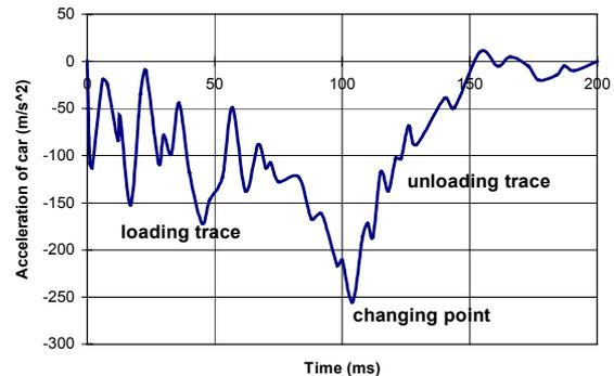
**Figure 7. Crash pulse of an 1830kg sedan impacting an energy absorbing underrun barrier system at 48km/h**
