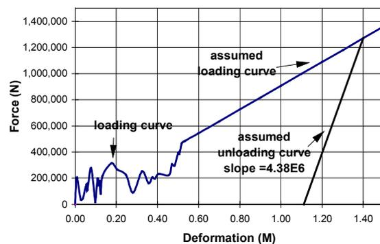
**Figure 9. Load-deformation curve of the car's front end determined from the crash test data shown in Figures 7 & 8.**
