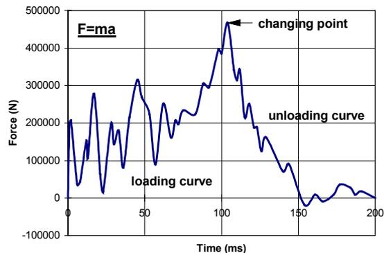
**Figure 8. Force-time curve of the car's front end derived from the crash pulse shown in Figure 7.**
