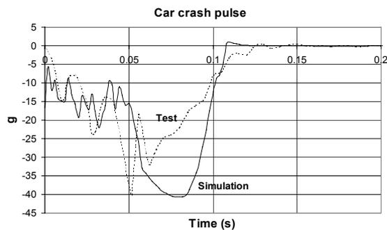
**Figure 12. Car crash pulse for the 1350kg sedan impacting at 75km/h into the energy absorbing rear underrun barrier system fitted to a 9.1 tonne truck.**
