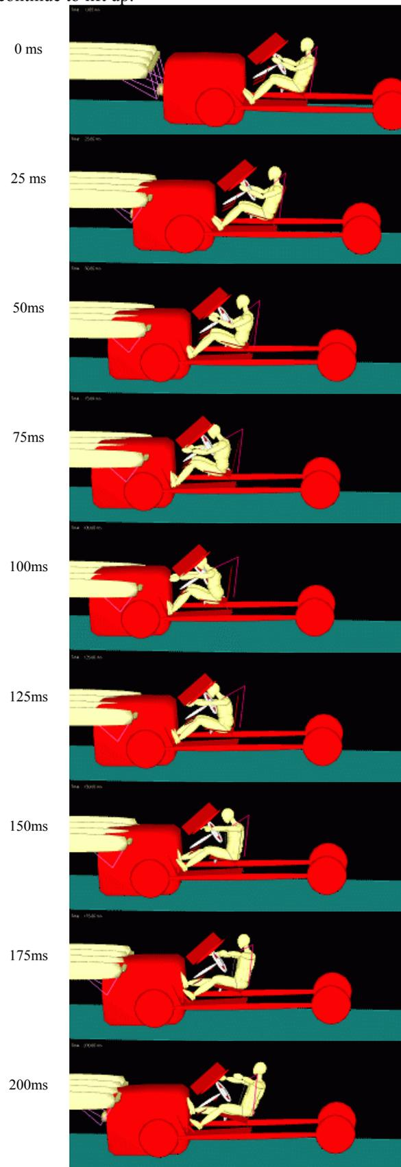
Figure 11. Kinematics of the 1350kg sedan impacting an energy absorbing underrun barrier system fitted to a 9.1 tonne truck at 75km/h.
