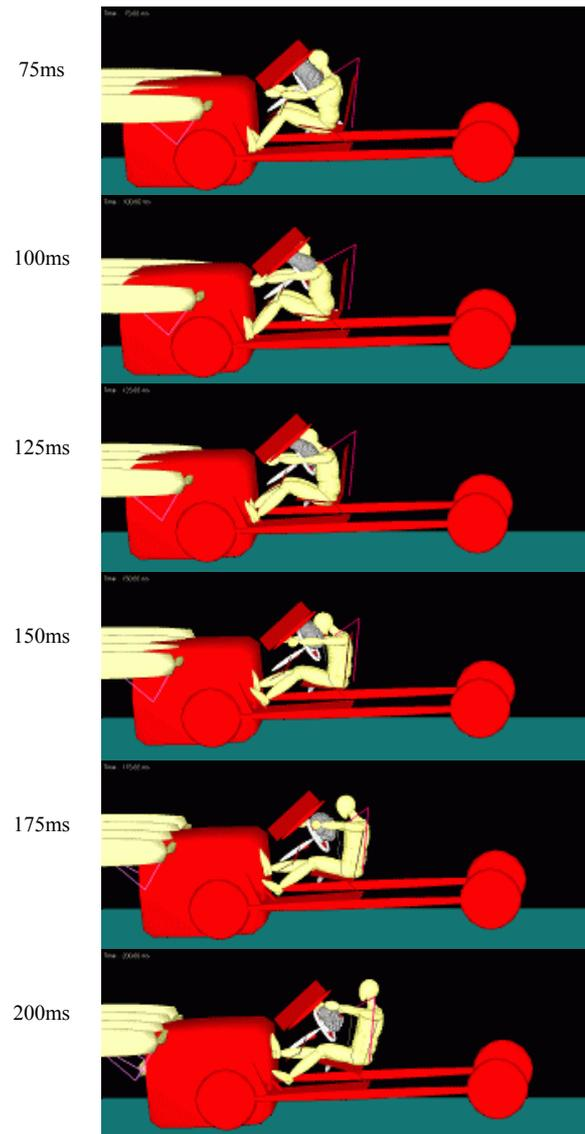
**Figure 12. Kinematics of an airbag equipped 1350kg sedan impacting an energy absorbing underrun barrier system fitted to a 9.1 tonne truck at 75km/h.**
