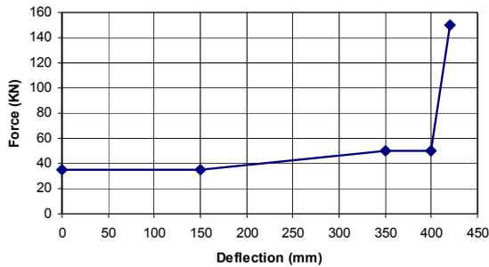
**Figure 6. Idealised force deformation curve of the energy absorbing unit used for the MADYMO model**
