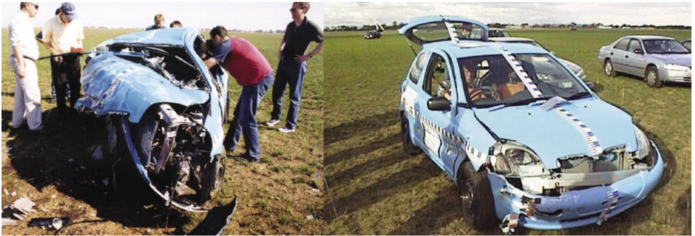
Figure 4 The difference in damage sustained by a small car impacting concrete barrier (left) and a wire rope barrier (right). The test involved the vehicle impacting the barriers at a speed of 80km/h at an angle of 45°.
